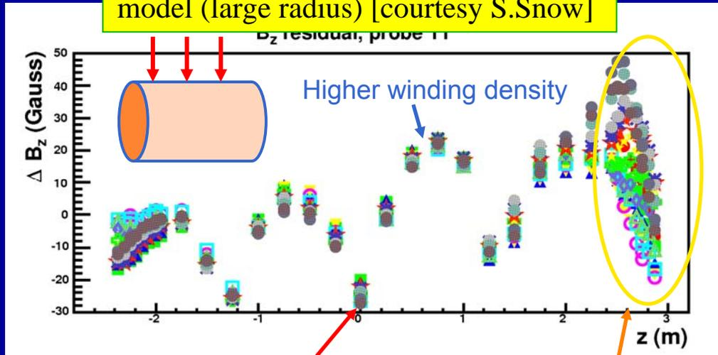
Conductor joint = missing 1 turn to be studied
