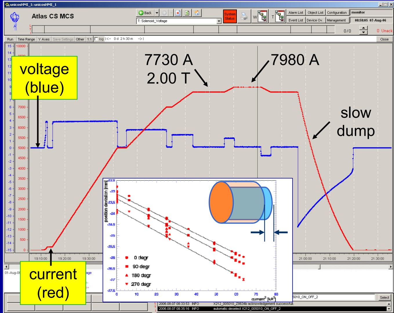
Coil length shrinkage, linear to  $I^2$
